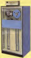
Loops of tape allow the stop/start to be unaffected by the inertia of the reels.
